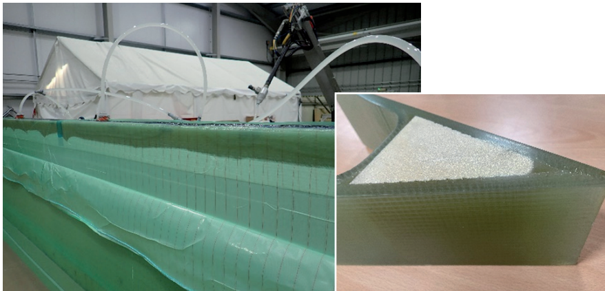
Above: Large infusions are an ideal application for PRIME™ 37 Right: An example of a complex laminate made with PRIME™ 37
