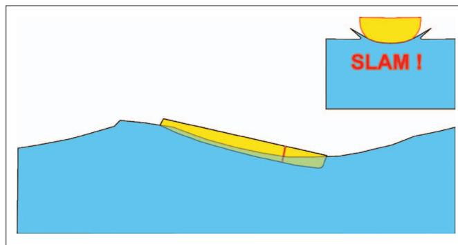
**Recorded vertical acceleration and typical attitude of the boat relative to the wave profile during a slamming event**
