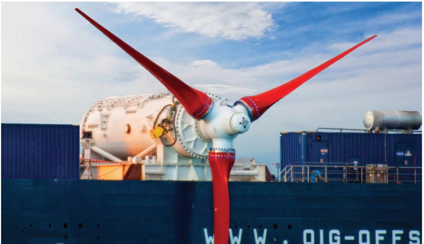
**With a rated capacity of 1MW and a diameter of over 20m the ANDRITZ HYDRO Hammerfest HS1000 is the largest single tidal turbine rotor to be installed to date. The 9m tidal blades were engineered and manufactured using Gurit materials by a team at Gurit UK.**
