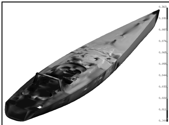
Figure 6: Strains on a yacht FE model subjected to the W1 equilibrium loadcase, sailing upwind on starboard tack. The strains on the foredeck are due to the global longitudinal bending moment from the rig. The highest strains on the deck are due to transverse compressive loads from the mast and chainplate bulkheads. The yacht is the Baltic 147, designed by Reichel/Pugh and engineered by SP Technologies.
